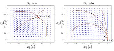
Fig. 4. 2D vector-fields of a two-node system illustrating locally controllable (Fig. 4(a)) and locally uncontrollable (Fig. 4(b)) overloads.
